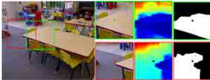
Fig. 2. Two examples to show inferred depths and activation maps (output from nonlocal correlation) from the marked color patches extracted within nonlocal neighborhoods.
